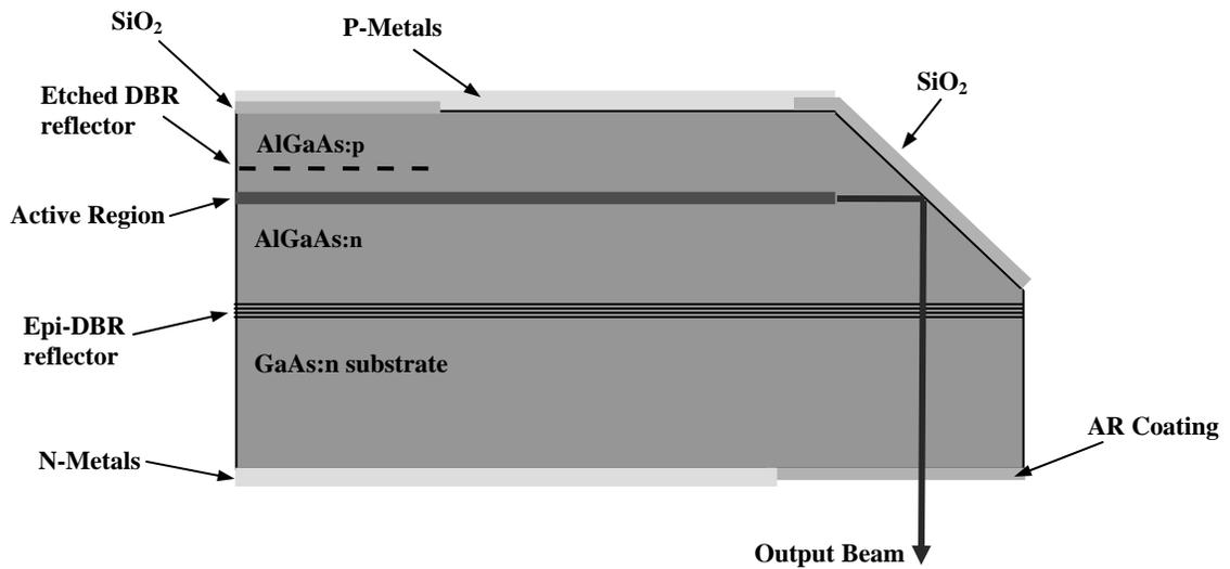
Figure1. Schematic diagram of vertical emitting laser chip.
