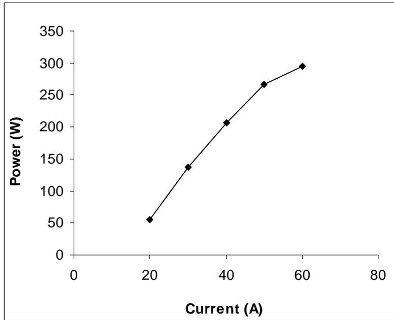
Figure 3. L-I characteristics from a 10x22 surface emitting array.
