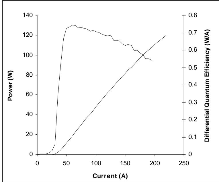
Figure 2. L-I characteristics from a 60 element 2-D surface emitting array.
