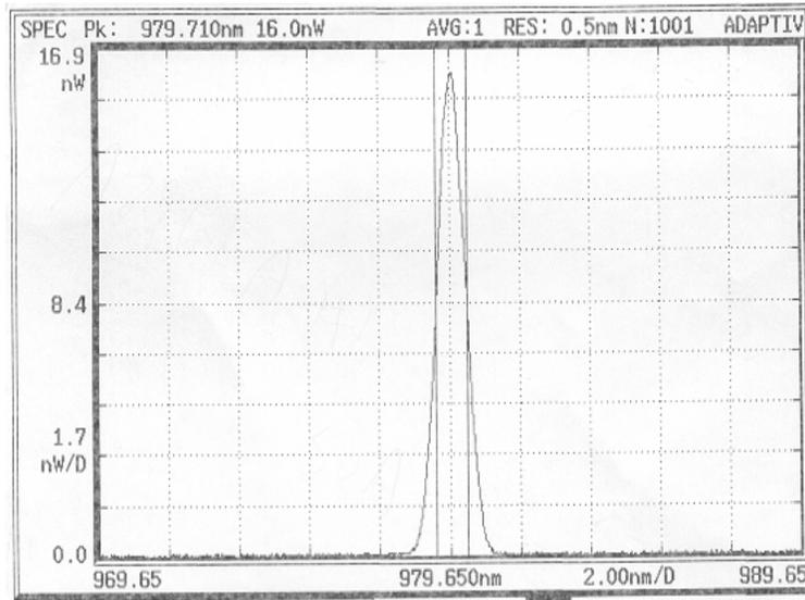
Figure 4. Optical spectrum from 10x22 array measured at 50 A. The full-width at half-maximum is approximately 0.9 nm.
