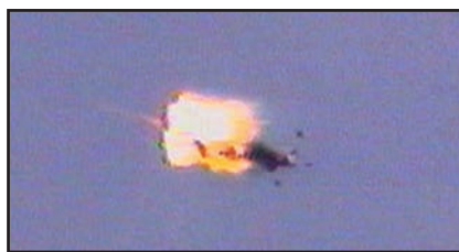
Figure 3. The US Army's Tactical High Energy Laser destroyed an armed Katyusha rocket in flight at the White Sands Missile Range in New Mexico in June 2000. The deuterium-fluoride chemical laser detonated the rocket's high-explosive warhead at a range of a few kilometers. Courtesy of Northrop Grumman Space Technology.
